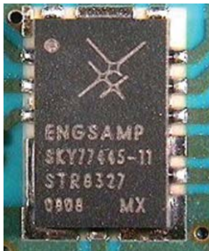
▲ Fig. 5 Packaged SKY77445 FEM utilizing Skyworks' multi-laminate substrate technology.
