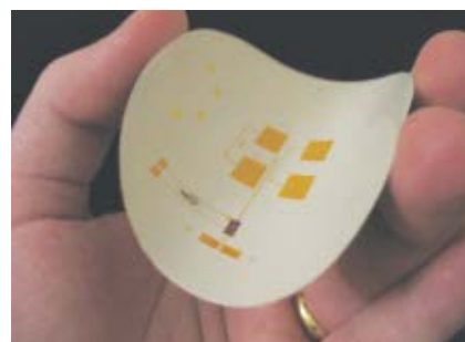
▲ Fig. 7 A completely flexible communication module fabricated on LCP.
