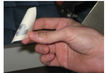
▲ Fig. 4 UWB antenna fabricated on LCP using a conductive printing technique.
